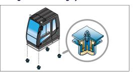
The application of Viscous Mounting to the cabin support provides the operator with a much improved ride. The operator work efficiency will increase as the shock and noise level in the cabin decreases.
