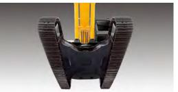
Reinforced box-section frame welded, low-stress, high-strength steel, guarantees safety and resistance against external impact when driving on rough ground and working on wet sites through high tensile strength steel panels, with highly durable upper and lower rollers and track guards.
