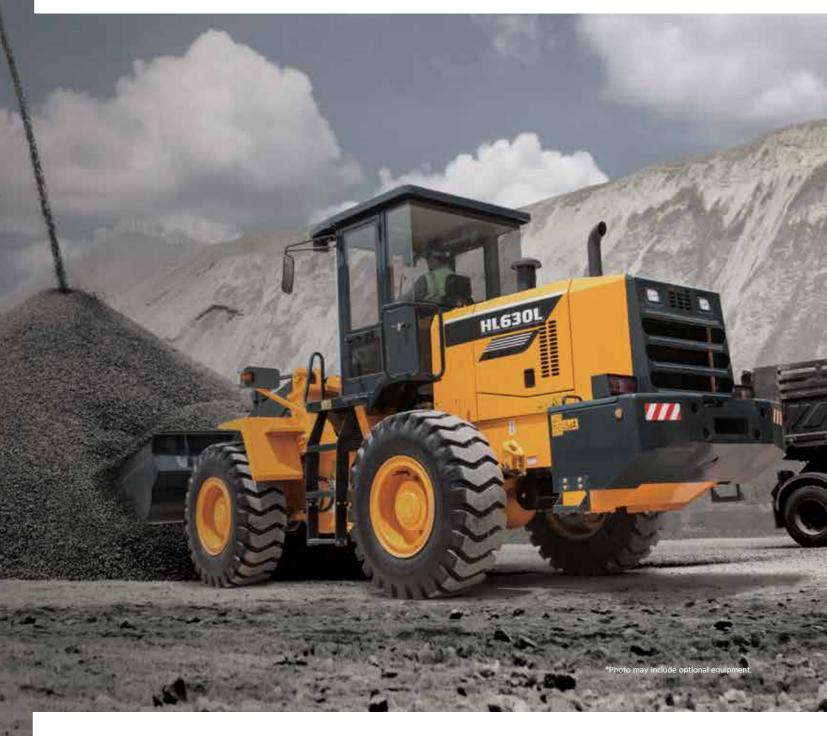
**Gross Power** 92 kW at 2,000 rpm Net Power 83 kW at 2,000 rpm **Operating Weight** 10,300 / 10,400 kg
